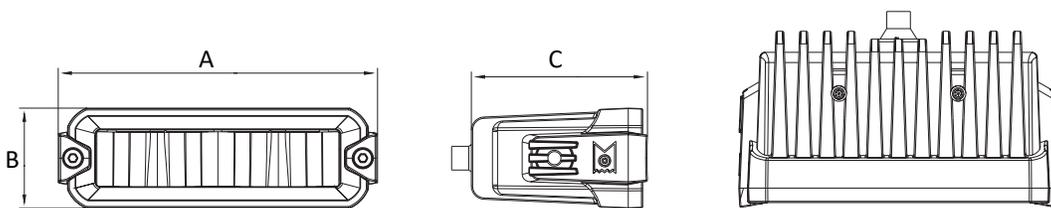
A: 4-<sup>3</sup>/<sub>4</sub>"    B: 1-<sup>1</sup>/<sub>2</sub>"    C: 2-<sup>1</sup>/<sub>2</sub>"
