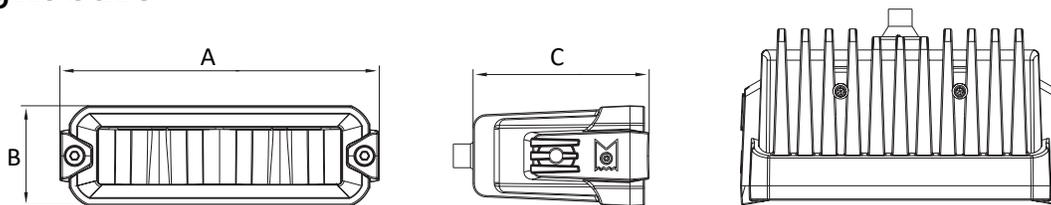
A: 4-<sup>3</sup>/<sub>4</sub>"    B: 1-<sup>1</sup>/<sub>2</sub>"    C: 2-<sup>1</sup>/<sub>2</sub>"
