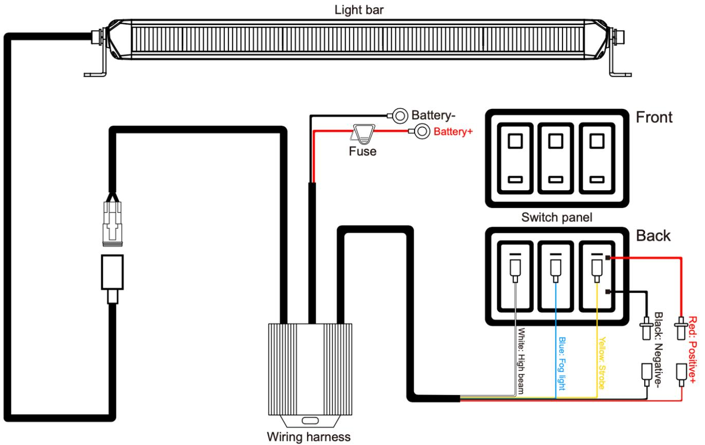
1. Determine suitable mounting locations to install the LED light bars, wiring harness and switch panel. Once all mounting locations are confirmed, connect the wires as shown above. Proper insulation at connections is required.
