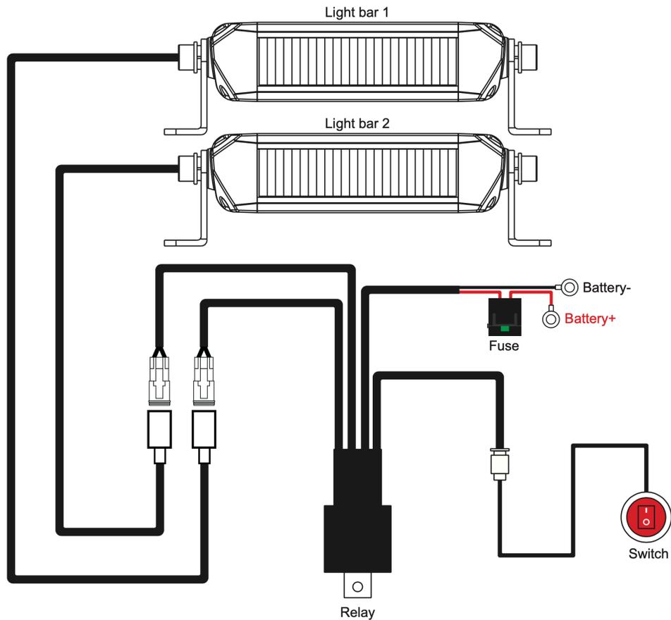
1. Determine suitable mounting locations to install the LED light bars, wiring harness and switch. Once all mounting locations are confirmed, connect the wires as shown above. Proper insulation at connections is required.
